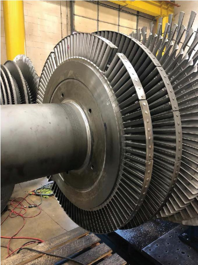
RTS received the rotor and an Engineered rotor modification package to follow for the stage 12 wheel and blade root modification. Stage 12 wheel faces and blade root were machined to new designed profile.
